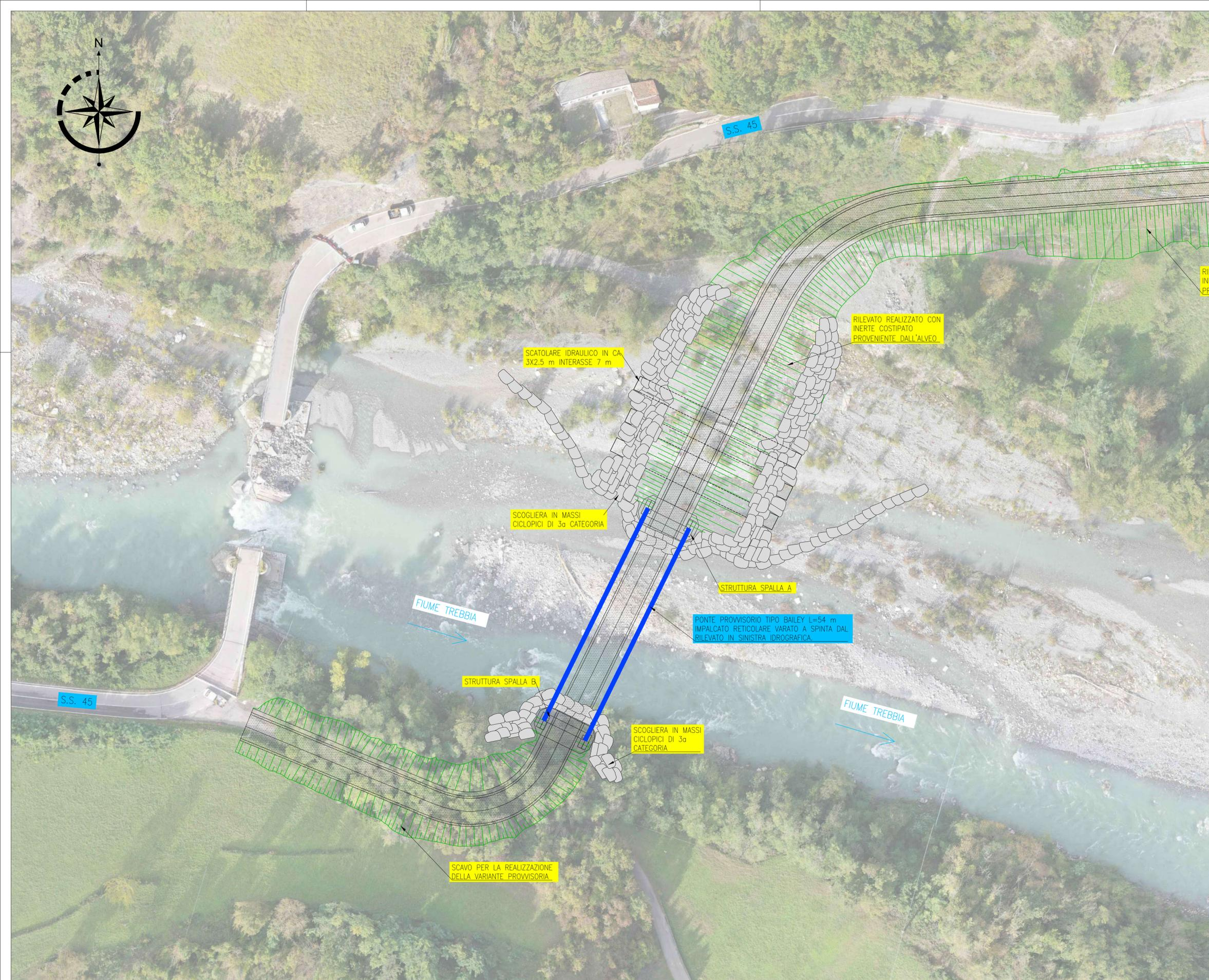
RILEVATO REALIZZATO CON INERTE COSTIPATO PROVENIENTE DALL'ALVEO.
